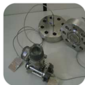
22,500 psi Tested DP Transmitters, GE
