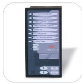
Alarm & Monitoring panel mounted on-board marine service
