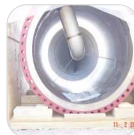
DN 60" V-Cone™ KOC Booster Station
