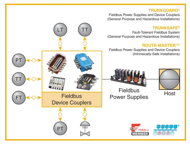
Fieldbus Device Couplers and Power Supplies deliver a fast and easy way to connect, protect, power and terminate multiple fieldbus devices in FOUNDATION fieldbus<sup>™</sup> and PROFIBUS PA segments.
