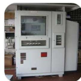
Zone 1 Eex p Calorimeter General Electric
